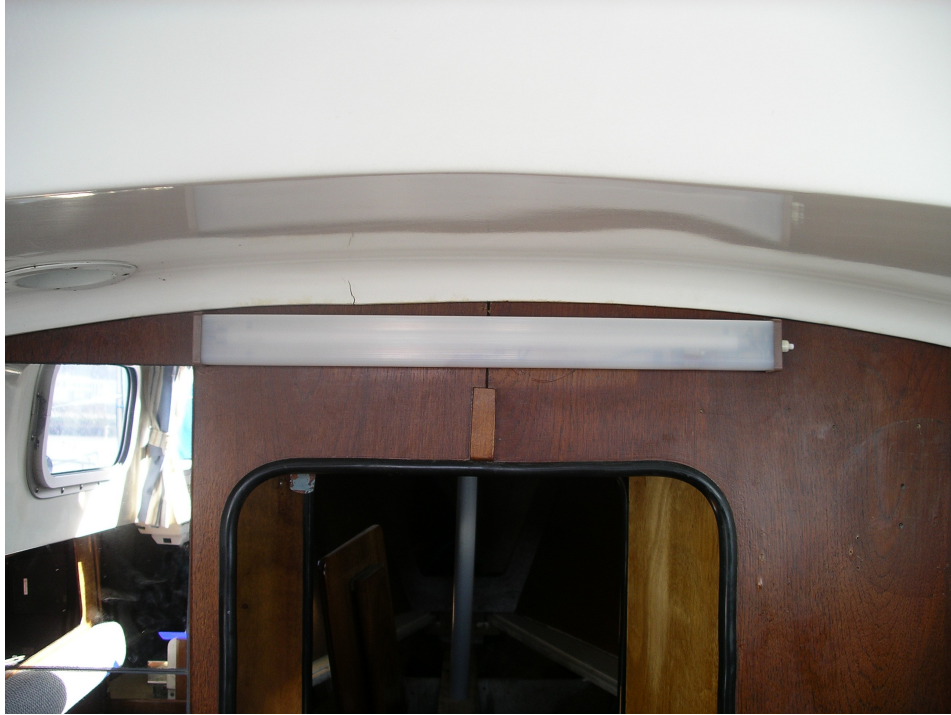
Photo 5389: crack to lining around 2 nd bulkhead
