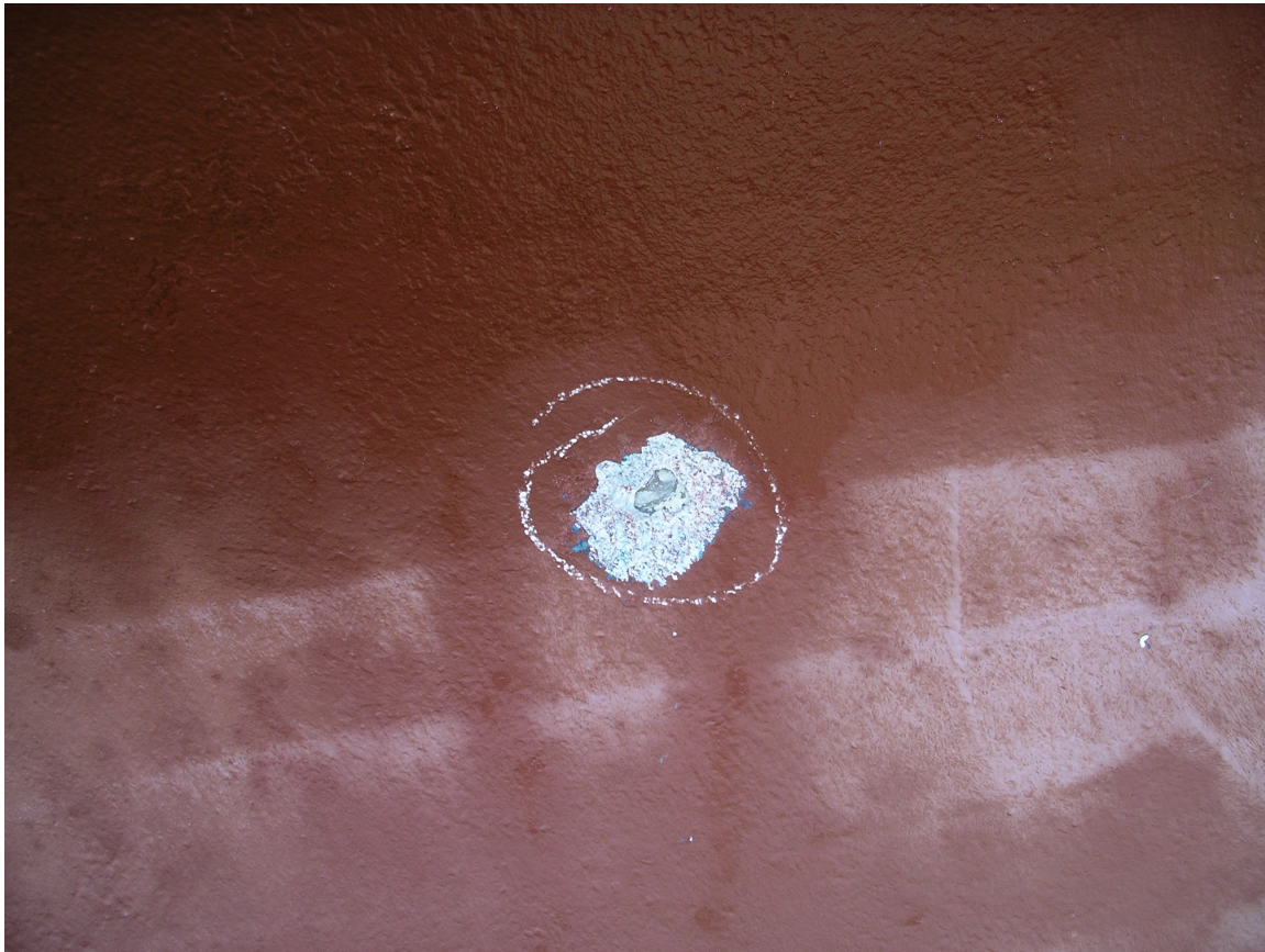
Photo 5386: area of epoxy failure on hull forward of propeller
